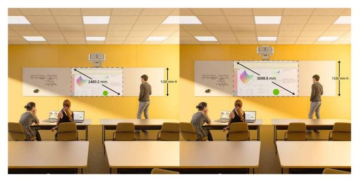
1219.2 mm 16:9 Ratio = Approx 1219.2 mm H x 2159 mm W = 2489.2 mm Diagonal (nominal) 1524 mm 16:9 Ratio = Approx 1524 mm H x 2692.4 mm W = 3098.8 mm Diagonal (nominal)
