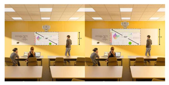
48 in 16:9 Ratio = Approx 48 in H  $\times$  85 in W = 98 in Diagonal (nominal) 60 in 16:9 Ratio = Approx 60 in H  $\times$  106 in W = 122 in Diagonal (nominal)
