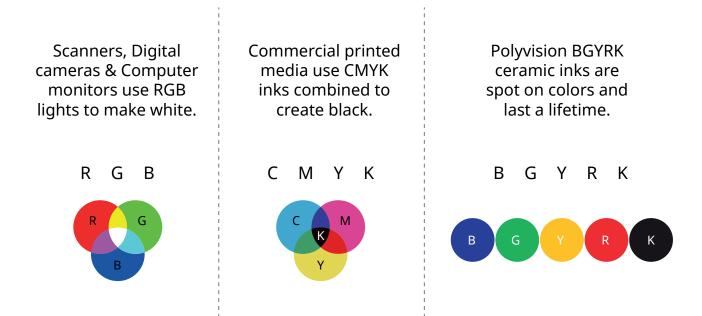
While a smaller color gamut for CeramicSteel printing when compared to CMYK devices, the pigmentbased ceramic inks fuse into the surface of the CeramicSteel sheet to create a permanently colorfast and durable surface unlike any other architectural panel product.
