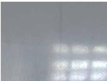
(loss of gloss and erasability -left- of a poor whiteboard surface – exaggerated test for illustration purpose)
